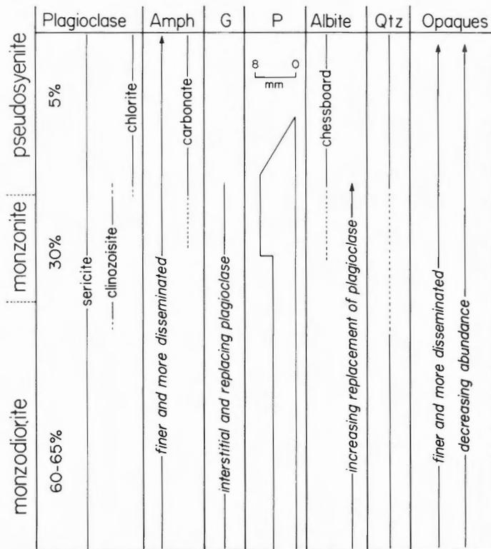
**Figure 37.** Diagram summarizing mineralogy of the Rainy Lake Intrusive Complex. Amph = amphibole, G = granophyre, P = perthite, Qtz = quartz.
