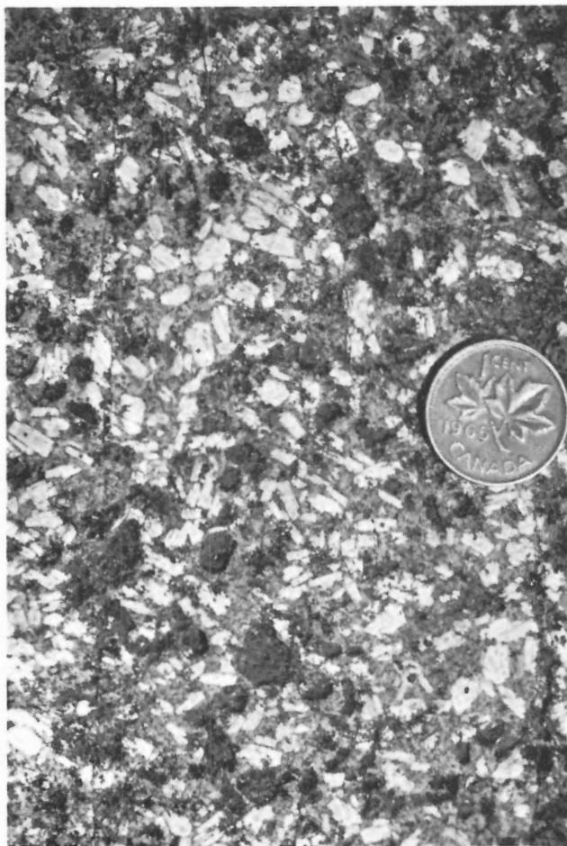
**Figure 39.** Detail of upper border monzonite, Rainy Lake Intrusive Complex, Terra Ridge. Note the similarities of plagioclase phenocrysts to those of andesites of the Camsell River Formation. (GSC 190538)
