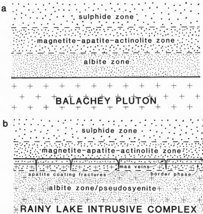
**Figure 43.** Comparison of alteration zoning between the Balachey Pluton (a) and the Rainy Lake Intrusive Complex (b). Note that the magnetite-apatite-actinolite zone occurs partly within the upper part of the Rainy Lake Intrusive Complex.
