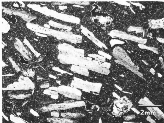
**Figure 24.** Photomicrograph of flow-oriented plagioclase phenocrysts in andesitic lava flow, Camsell River Formation. (GSC 190595)
