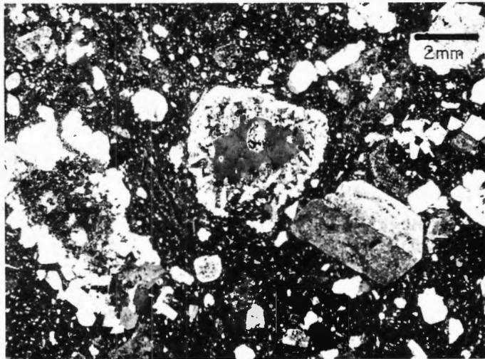
**Figure 57.** Clinopyroxene armoured quartz xenocrysts (centre), altered K feldspar xenocryst, and clinopyroxene clots, Animal Andesite. (GSC 190611)
